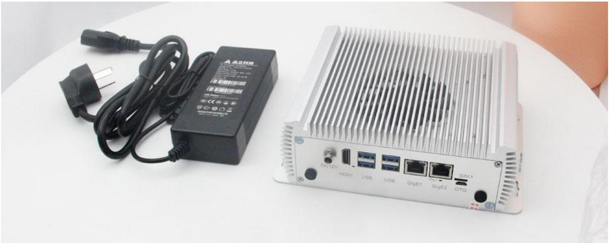
The 11F1E2 AI Computing Platform (hereinafter referred to as 11F1E2) is compatible with the NVIDIA Jetson Orin NX/ Orin Nano core module. Can provide up to 100 TOPS computing power, with a wealth of external interfaces, internal interface devices are wide temperature models.
